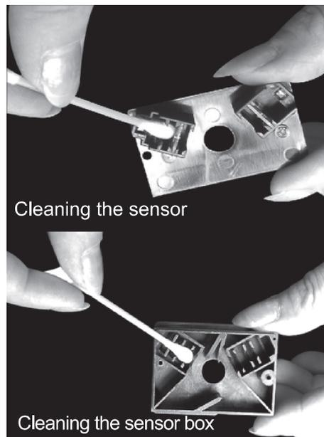
5. Put back the sensor correctly after cleaning, make sure that the cord is reconnected in the correct direction.
